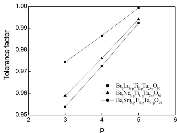
Fig. 2. Tolerance factor ( $t$ ) of tungsten bronze compounds  $\text{Ba}_p\text{Ln}_{6-p}\text{-Ti}_{8-p}\text{Ta}_{2+p}\text{O}_{30}$  ( $\text{Ln} = \text{La}, \text{Nd}, \text{Sm}$ ) as function of composition  $p$ .
