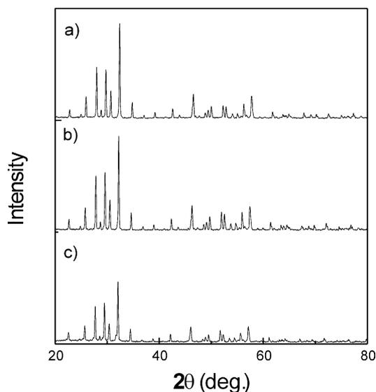
Fig. 1. XRD patterns of (a)  $\text{Ba}_3\text{La}_3\text{Ti}_5\text{Ta}_5\text{O}_{30}$ , (b)  $\text{Ba}_4\text{La}_2\text{Ti}_4\text{Ta}_6\text{O}_{30}$  and (c)  $\text{Ba}_5\text{LaTi}_3\text{Ta}_7\text{O}_{30}$ .
