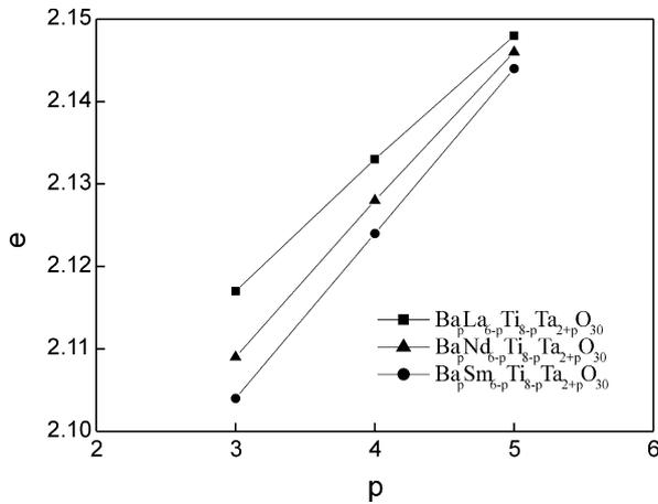
Fig. 3. Average electronegativity difference ( $e$ ) of tungsten bronze compounds  $Ba_pLn_{6-p}Ti_{8-p}Ta_{2+p}O_{30}$  ( $Ln = La, Nd, Sm$ ) as function of composition  $p$ .
