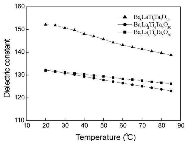
Fig. 5. Variation of dielectric constant with temperature at 1 MHz:  $\text{Ba}_3\text{La}_3\text{Ti}_5\text{Ta}_5\text{O}_{30}$  sintered at  $1425^{\circ}\text{C}$ ;  $\text{Ba}_4\text{La}_2\text{Ti}_4\text{Ta}_6\text{O}_{30}$  sintered at  $1400^{\circ}\text{C}$ ;  $\text{Ba}_5\text{LaTi}_3\text{Ta}_7\text{O}_{30}$  sintered at  $1425^{\circ}\text{C}$ .
