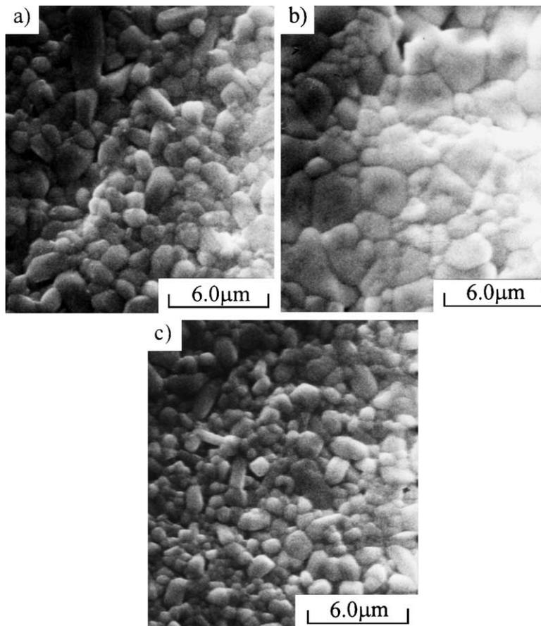
Fig. 4. SEM micrographs of polished and thermal-etched surfaces of (a)  $\text{Ba}_3\text{La}_3\text{Ti}_5\text{Ta}_5\text{O}_{30}$ , (b)  $\text{Ba}_4\text{La}_2\text{Ti}_4\text{Ta}_6\text{O}_{30}$  and (c)  $\text{Ba}_5\text{LaTi}_3\text{Ta}_7\text{O}_{30}$  ceramics.
